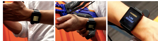
Figure 5-16. Augmenting analog experiences. In Nerf gun, we can detect users loading ammo clips (left) and firing darts (middle).
