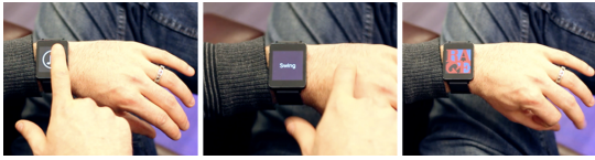
Figure 5-11. In a launcher, we can place navigation controls on the skin. Users can traverse back up through the hierarchy with a flick gesture.
