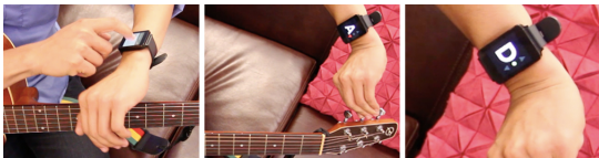
Figure 5-15. For an unpowered object e.g. , an acoustic guitar, we can detect the closest note to tune the instrument precisely.
