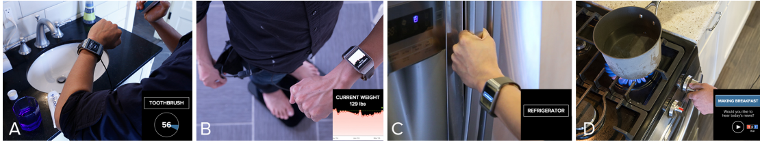
Figure 4-6. EM-Sense can augment activities in the home. For example, EM-Sense can launch a timer (inset) when the user is brushing his teeth (A), or display the user’s data when stepping on a scale (B). Next, EM-Sense knows that the user is making breakfast and fetches the morning news (C and D).
