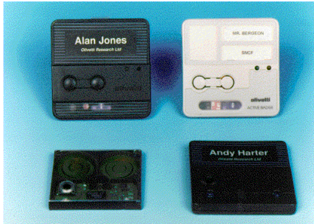
Figure 2-1. The Active Badge prototype, one of the earliest context-aware systems
