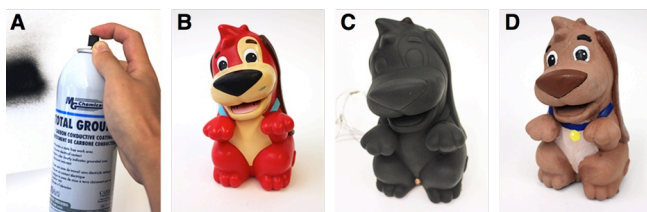
Figure 5. We carbon sprayed (A) an off-the-shelf toy (B) to make it interactive. A new topcoat was applied (C to D).
