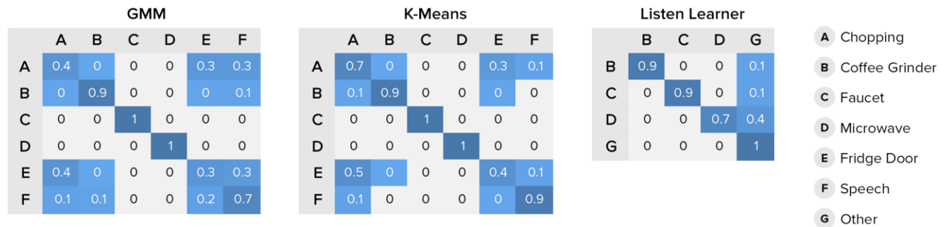
Figure 6. Visualization of the different sources of error for GMM (left), K-Means (center), and Listen Learner (right) in the Apartment Kitchen environment. True labels are listed on the y-axis and predicted labels are on the x-axis. Note Listen Learner contains fewer classes because classes below a confidence threshold are ignored. The “other” category consists of classes not yet discovered by Listen Learner, which are ignored.
